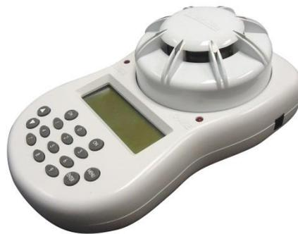
The MKII Handheld Programmer is designed to complement all MKII devices and to assist the commissioning engineer on site. The unit will softly address all devices without using the incorporated dip-switch on the field devices. Smoke and heat detectors can be tested when plugged on the programmer and alarm LED's can be verified prior to installation. The MKII Programmer can also re-program the OPT-HEAT detectors to either heat or smoke detector.
