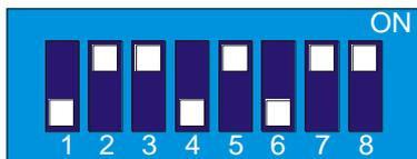
The Address setting is binary, with the ON position being binary 0, and the OFF position being binary 1
