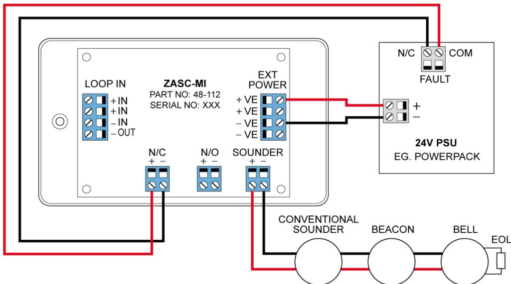
The ZASC requires an external 24vdc power supply (as shown in the above diagram). The EOL for the sounder circuit is 4K7 Ω. When using the ZASC make sure the PSU being used has a fault output relay, so that in the event of a power supply fault it is reported to the control panel.
