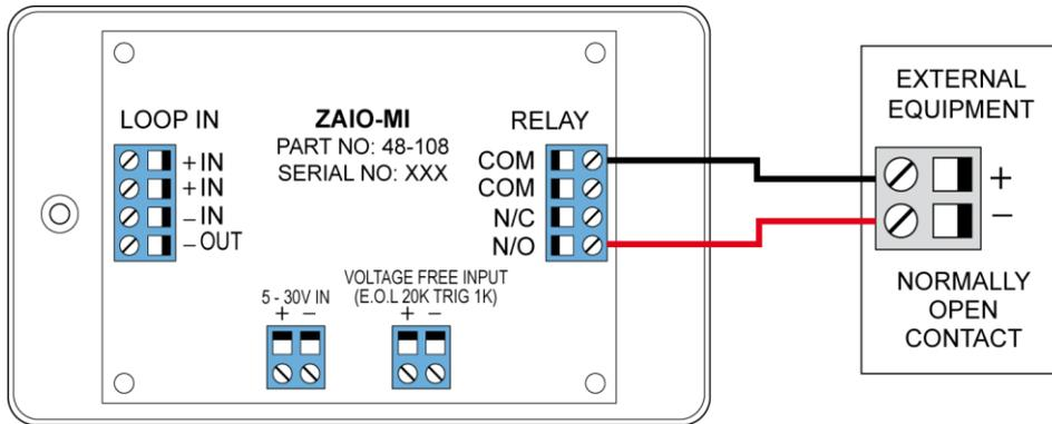
The end of line resistor value is 20KΩ and the trigger resistor value is 1kΩ.
