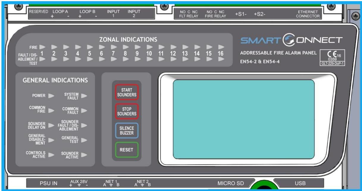
The panel contains the following mandatory controls. They can only be operated when the user or engineer (ADMIN) password has been entered. The CONTROLS ACTIVE LED indicates that the controls have been enabled.
