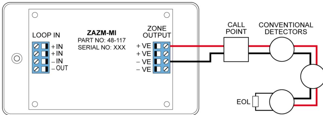
The ZAZM powers the conventional zone from the addressable systems loop, so no external power supply is required. The EOL for the zone is 6.2KΩ.
