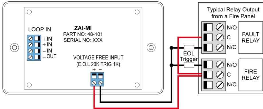
The end of line resistor value is 20KΩ and the trigger resistor value is 1kΩ.
