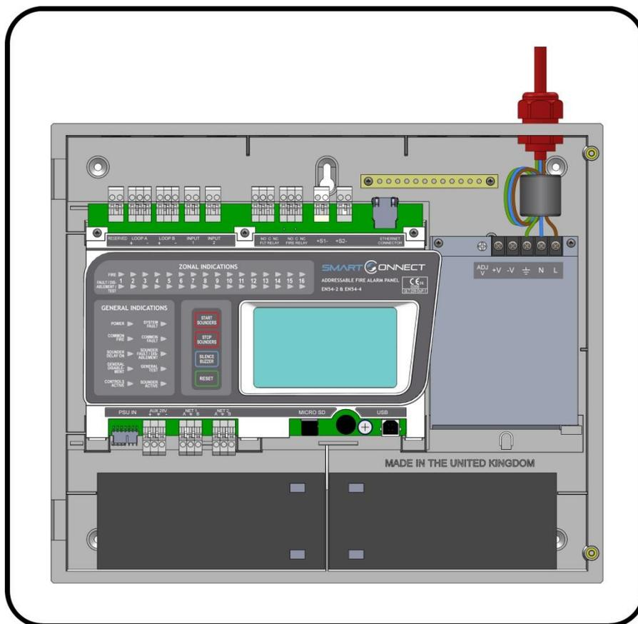
Figure 2: Wiring the mains connection
