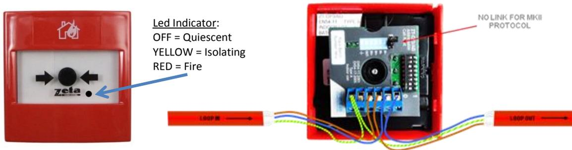
The CP3/AD call point has a built in isolator which can be wired in circuit or not used. This is done by means of not wiring to the negative out terminal on the call point. The following terminals are used for connecting the call point.
