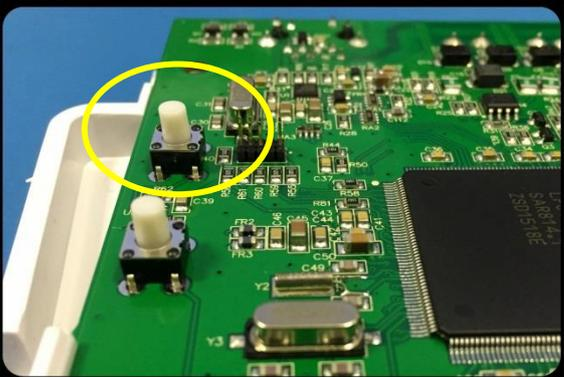
A photograph of the rear of the PCB. The PCB is green. A small, round, white button is visible on the PCB, circled in yellow. The button is mounted on a small metal base. Various electronic components are visible on the PCB.                                                                                                                   |
