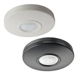
The ceiling mount, low profile panoramic DS936 PIR Detector uses alternate polarity pulse count. It also uses a Fresnel lens to provide up to 7.5 m (24 ft) of coverage and can be mounted on the surface, or semi-flush directly to a ceiling or a standard octagonal electrical box.
