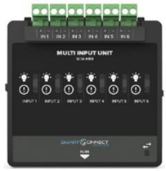
The SCM-MIM has six class B inputs that are commonly used to monitor and raise alarms from any specific ancillary equipment.
