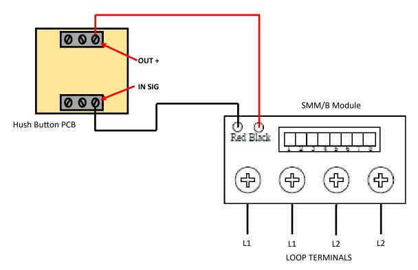
Note: Loop L1 and Loop L2 are polarity insensitive, but, for the sake of consistency, it is recommended that Loop L2 be kept positive.
