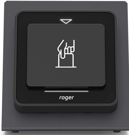
RUD-4-DES is a desktop reader and writer for MIFARE® Classic, Plus (S, X) and DESFire (EV1, EV2, EV3) cards which also allows reading an EM 125 kHz standard proximity cards. It is supplied directly from a USB serial port, which is also used for communication with the PC. The device has a stable metal desktop stand with a card holder. The RUD-4-DES can be used as a card enrol reader for the access control system or any other application which requires a card reader. A card can be enrolled
